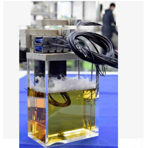
A palm-size automatic beer brewing machine developed by Takasago Electric Inc.
